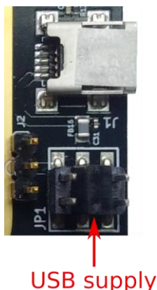
Figure 4.2: Setup for USB supply for LMS8001 CMP
