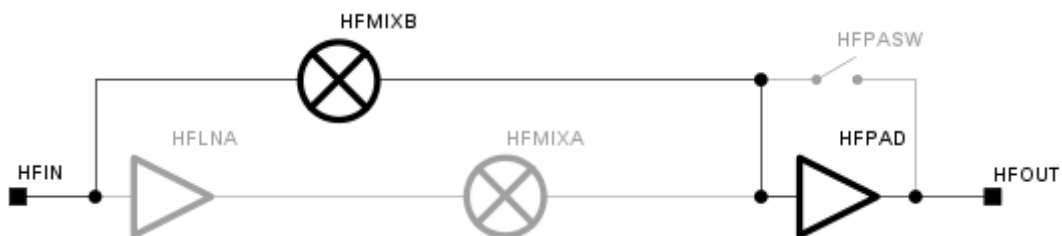
Figure 3.5: Example of up-conversion channel configuration
